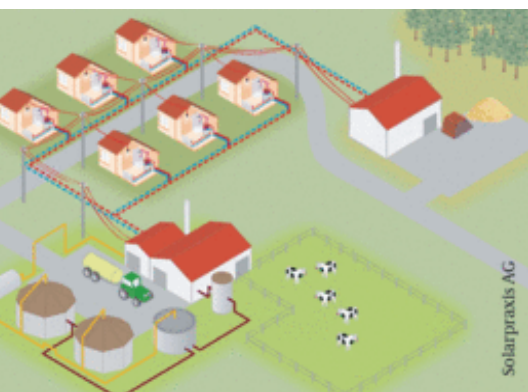
Figure 7: Schematic diagram of biogas use to generate electricity and heat.
